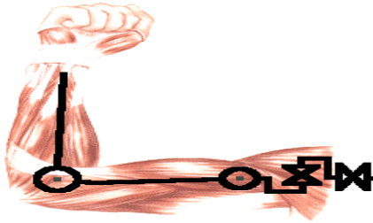
Fig. 2. Analogy Human Hand to 2- Links Mechanism
