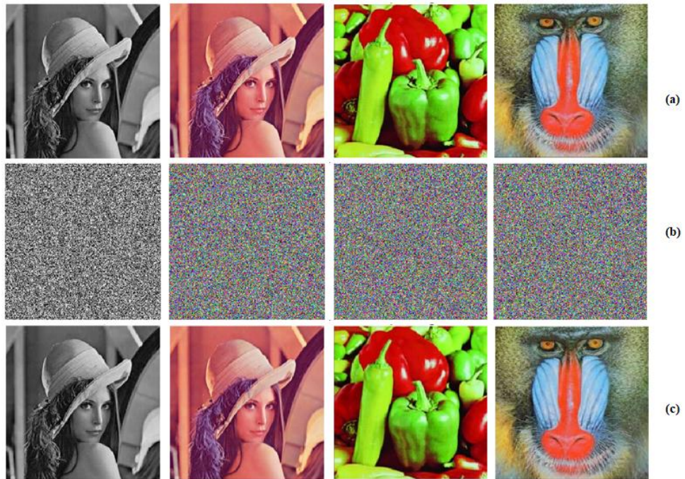
Fig.3. Encryption Results for Various Images (a) Original images; (b) Images encrypted with the proposed algorithm; (c) Decrypted images. (From right to left: Baboon, Peppers, color Lena, and grayscale Lena).
